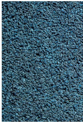
POURED-IN- PLACE (PIP) RUBBER SURFACING
