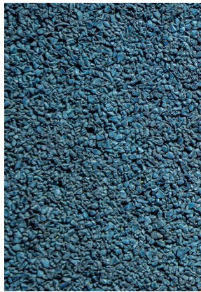
POURED-IN- PLACE (PIP) RUBBER SURFACING
